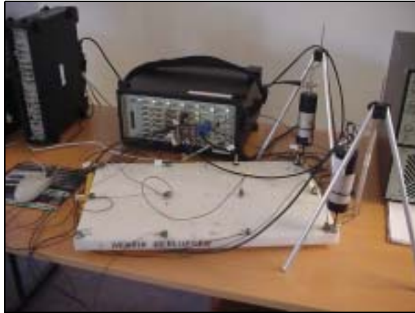
Fig. 17 Plate structure which exhibits two modes (torsional and bending) at (almost) the same frequency.
